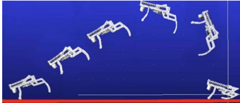
Figure 8. Bionic frog jumping trajectory
