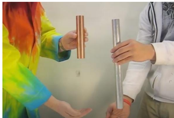
Figure 2. Picture of the experiment of a magnet falling in copper and aluminum tube [8]
