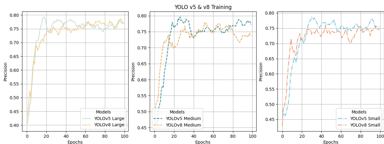
Figure 1. Performance comparison of large, medium, and small models within the YOLOv5 and YOLOv8 architectures for object detection task
