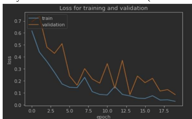
Figure 6. The loss curve of MobileNet + SE Block (Photo/Picture credit: Original).
