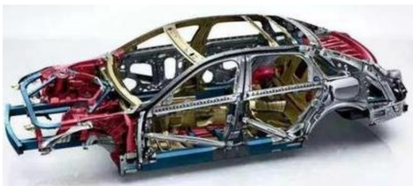
Fig 1. The main steel structure of a car [1].
