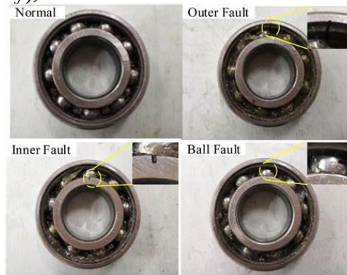
Figure 2. Bearing Fault Illustration
