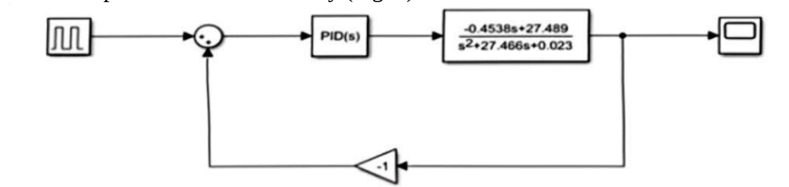
Fig. 2 Simulation of PID controller with Simulink [9]
