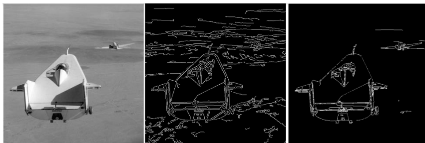
Figure 1. (a) Original Image (b) Traditional Canny Algorithm (c) Method for Images with Less Edge Information [4]
