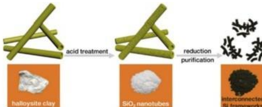
Fig 2. The preparation process of nano-silicon anodes [8].
